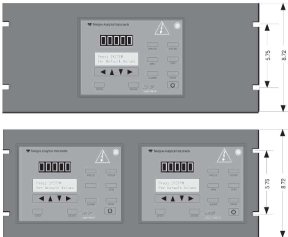
Figure 3-2: Single and Dual 19" Rack Mounts
